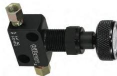
**Screw Type Proportioning Valve**, can be used effectively with single or dual master cylinder systems, providing better front-to-rear brake balance under both light and heavy braking. 90-2000 (AN-3) / 90-2003 (10mm)
