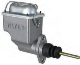
Designed for applications that require large fluid capacity in a leak-proof integral reservoir. These cylinders are also unique in that they may be temporarily inverted without loss of fluid. Fluid chamber is completely sealed from the outside environment while still allowing fluid level changes. Available in the most popular bore sizes, these cylinders are an affordable solution for the budget racer.
