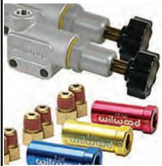
Wilwood offers both knob and lever style proportioning valves with varying in/out ports 1/8-27NPT, M10x1 BF, or 3/8-24IF. They also offer residual pressure valves in 3 color coded sizes 2, 4, or 10lb with or without fittings.
