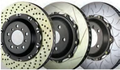
Upgrade and replace your heavy 1-piece rotor to a lightweight 2-piece disc system: comprised of an aluminum bell and outer iron disc with floating mounting hardware. These assemblies are direct OE replacements that work directly with stock calipers, and allow you to fine tune your systems initial bite characteristics and disc wear.
