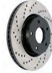
Cross Drill - Typically one hole per vane in a directional pattern. Assists cooling of the rotor while also releasing the gases. Not ideal for track use as it does lessen the surface area and makes it more prone to cracking.
