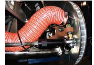
NEOPRENE 350°F - Designed for moving air from -65°F to 350°F, this Neoprene hose is an extremely lightweight, highly flexible, low pressure ducting. Constructed with fiberglass cord, bronze-plated steel-spring wire helix and rubber-coated fiberglass fabric to meet your ducting needs. Can be screwed together to form a continuous length. Perfect for air ducts, oil, and transmissions coolers. Comes in 10' sections.
