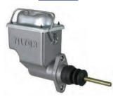
Designed for applications that require large fluid capacity in a leak-proof integral reservoir. These cylinders are also unique in that they may be temporarily inverted without loss of fluid. Fluid chamber is completely sealed from the outside environment while still allowing fluid level changes. Available in the most popular bore sizes, these cylinders are an affordable solution for the budget racer.
