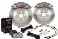
The Trophy Sport Big Brake kits are designed for street driven production vehicles and use the same STR caliper, AeroRotors and AeroHats as the Trophy Race kits but add silicone dust boots to extend service intervals and anti-rattle rotor mounting hardware for quieter street operation.
